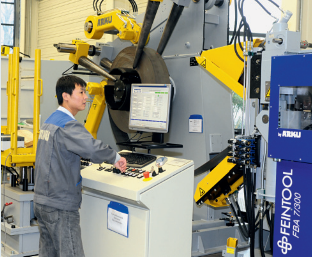
Service technician Mickey Li operates the coil feeding line
