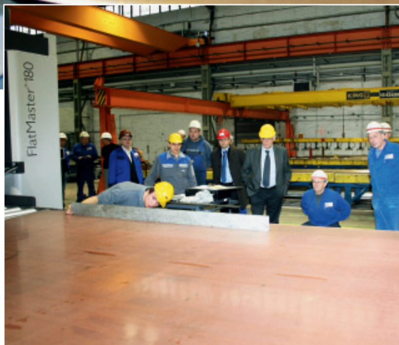
After leveling: flat and stress-free
